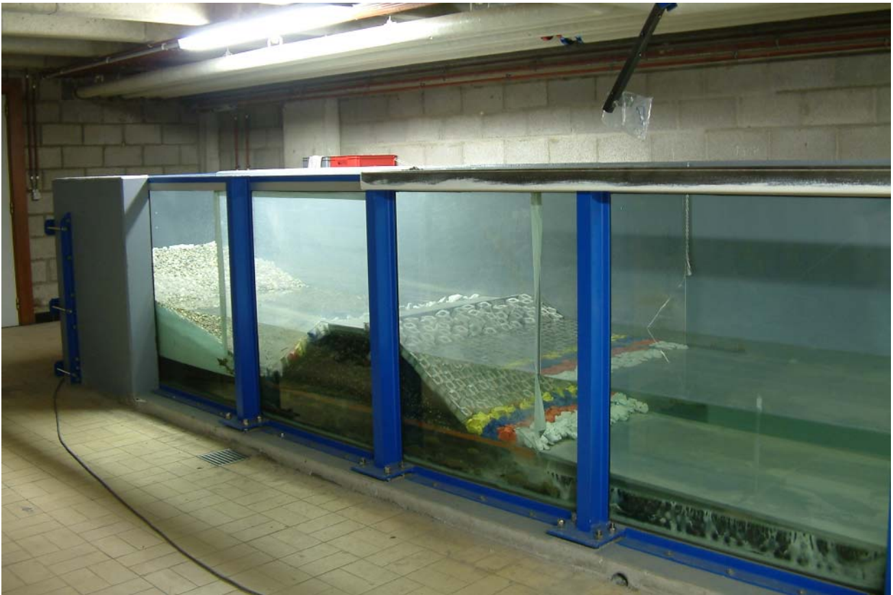
Figure 2: Model section with glass wall of the Large Wave Flume at Ghent University.
